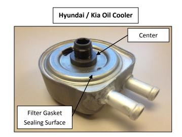
Oil leakage may occur if the oil cooler center bolt should loosen (see image above). This is possible after multiple filter changes. This may result in oil leakage incorrectly diagnosed as a filter leak. Consult with Hyundai/Kia Dealer or Service Manual for proper repair and installation instructions if center bolt is loose.
